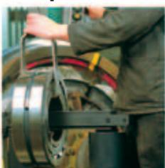
Mount workpiece either standing or lying on one side. Large workpieces are no problem with the 4x swivel arm.
