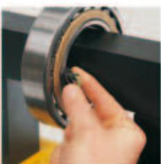
Mount the miniature magnetic temperature probe.
