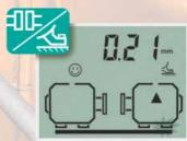
The alignment condition is displayed with a smiley, foot correction values, coupling gap and offset.
