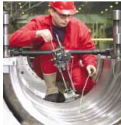
BORALIGN® & CENTRALIGN® – alignment of bores & turbines
