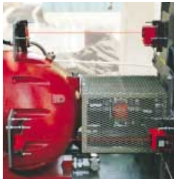
PERMALIGN® – continuous alignment monitoring
