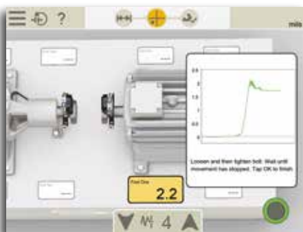
Soft Foot check on both machines.
