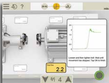
Soft Foot check on both machines.
